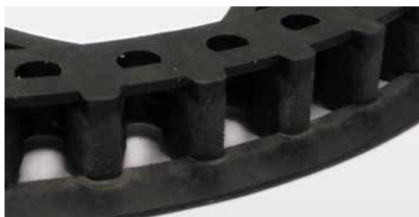
Signs of wear on a CDS eco sprocket
