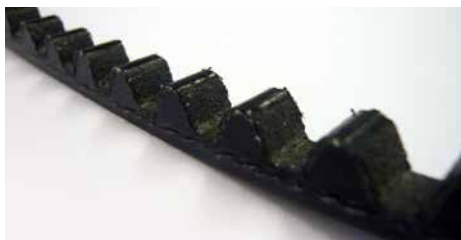
Signs of wear on the drive belt
