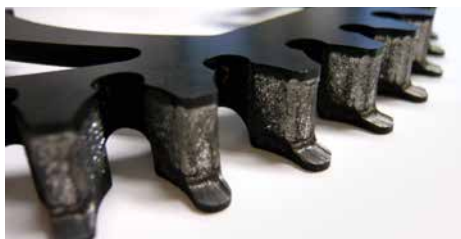
Signs of wear on a CDS premium or cargo sprocket
