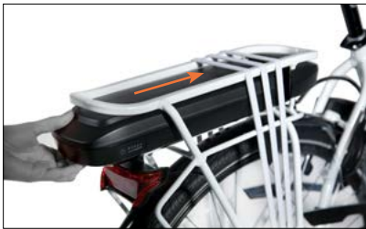
Fitting carrier battery
