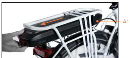
Removing carrier battery
